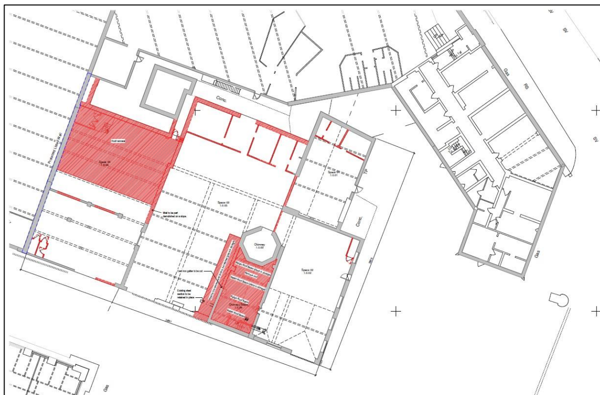
Image 9.1: Completed demolition works (removed fabric identified in red)
