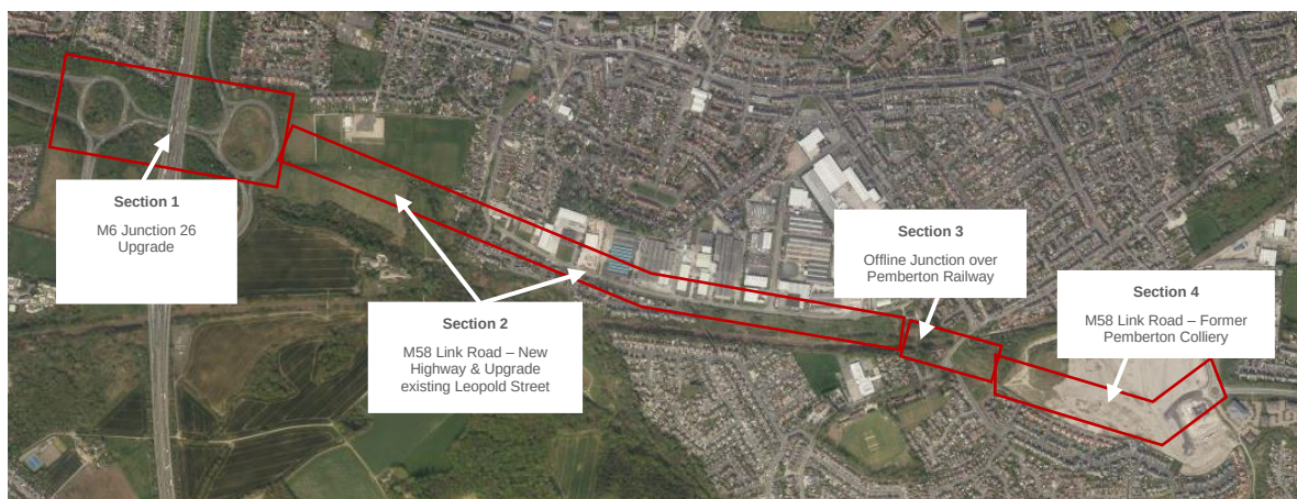
Figure 1-1 - Overview of scheme sections
